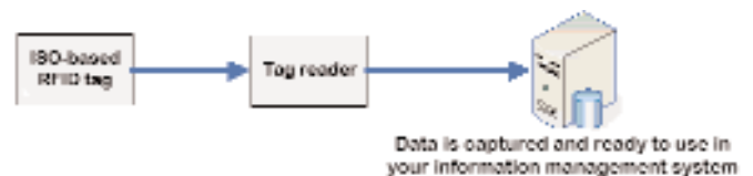
Figure 8 -The ISO approach is based on simplicity and direct access to information. The ISO tag is self-contained with all required information.
